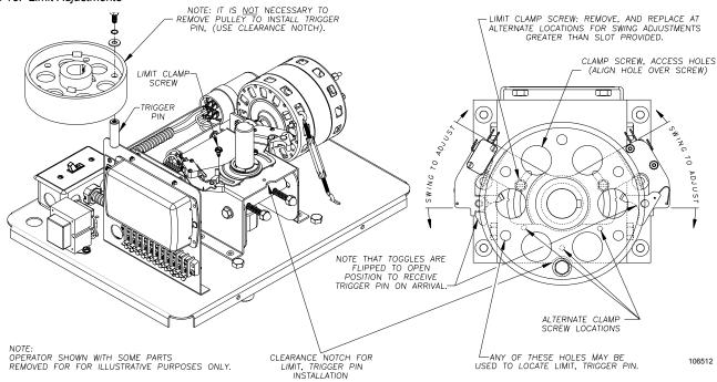
mounting hole is positioned directly above the clearance notch provided in the shaft support tower (see Figure 18). This notch provides the appropriate clearance to install the limit trigger pin with the bolt and washers provided. Install the trigger pin firmly in place.
